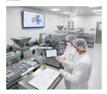
2. **Verify availability of new format parts:** Check that all required format parts (e.g., forming plates, sealing tools, feeders, guiding components, and change parts) are available, cleaned, and in good condition. Inspect for any wear or damage that could affect product quality or machine performance.
